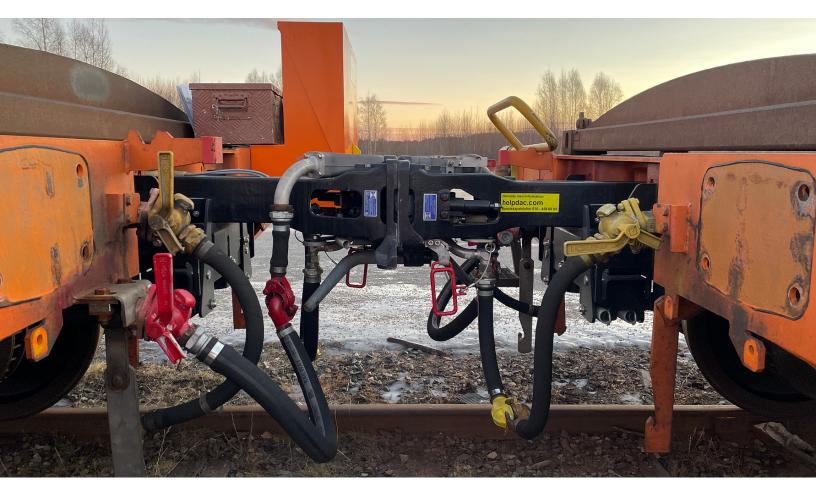
Digital automatic couplers are now being tested in the steel shuttle operated by Green Cargo for SSAB. Photo: Maria Lindholm/Green Cargo
